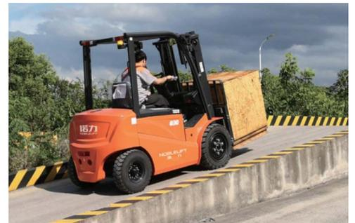
It is equipped with a powerful parking brake, enabling it to park with a load on a 15% gradient in complete safety.
