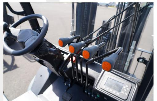
The U-shaped design of the steering wheel and the front-mounted multi-directional valve control make driving easy and effortlessly.
