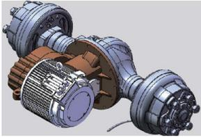
The transmission system uses a horizontal drive axle with a high gear ratio. The battery is installed at the bottom of the chassis. The trucks are equipped with a maintenance-free AC motor.
