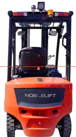
**C.** The Q series trucks are equipped with LED lights as standard, Blue spot, USB ports<sup>1</sup>, rear handle with integrated horn<sup>2</sup>. The aim is to offer the operator the greatest possible comfort and optimum safety in use.
