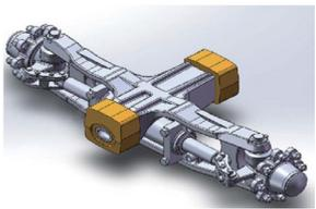
Fitted as standard with a steering axle designed to reduce vibrations. This design, with its flexibility, protects the trolley and extends its service life.
