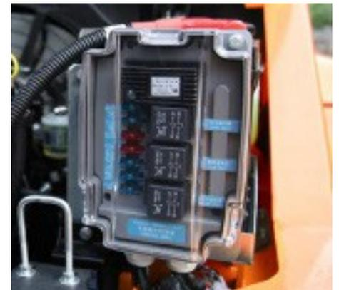
The controller, which incorporates all the electrical components, is protected from temperature, water and vibration by a special, easily accessible casing.
