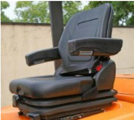
Operator presence system (OPS) - When the operator is not in the driver's seat, the hydraulic controls are activated. The lifting and tilting mechanisms lock automatically and travel is disabled.
