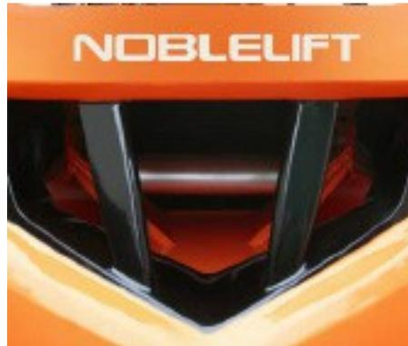
The optimised heat dissipation channel allows a larger radiator to be used, ensuring reliable engine operation even in the most demanding applications.
