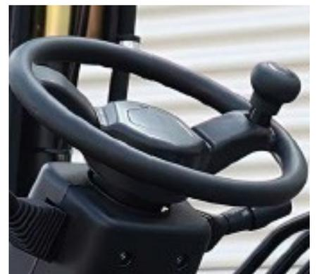
Fully hydrostatic power steering (FHPS) on demand ensures smooth, precise steering.
