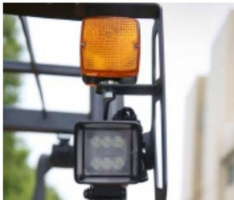
Equipped with LED lamps as standard: rear work lights, headlights, strobe lights and blue LED safety lights. Standard lighting provides optimum visibility and safety.
