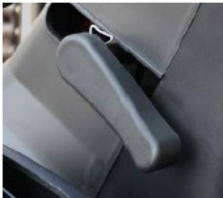
The angle of the steering column is easily adjusted using a lever on the left-hand side of the steering column.
