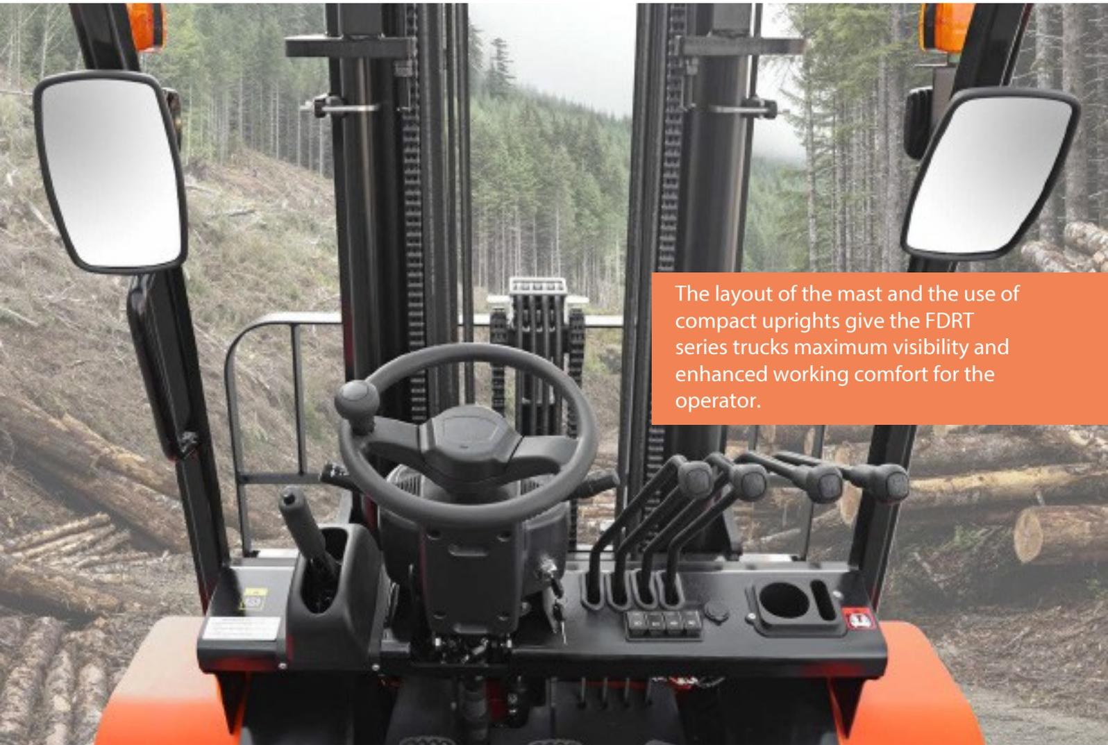
The layout of the mast and the use of compact uprights give the FDRT series trucks maximum visibility and enhanced working comfort for the operator.
