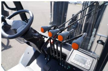
The Q range of electric trucks is fitted as standard with a new ergonomic steering wheel with a reduced diameter and a steering wheel ball. The truck is also equipped with a front multidirectional valve control, making work more comfortable.
