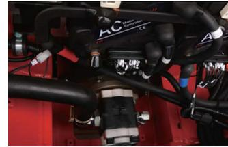
The traction motor is located high up, which makes it possible to make this trolley safe to use outdoors, particularly in damp environments.
