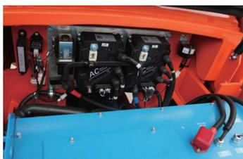
On the FE4P25Q-35Q model, the drives are positioned high up for efficient ventilation and easy maintenance.
