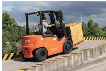
It is fitted with a parking brake. This high-performance vehicle can park safely on a 15% gradient with its load.
