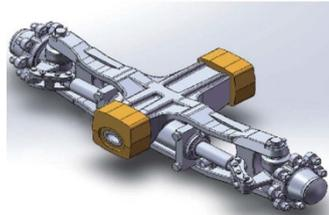
Equipped with a forged steering axle and shock-absorbing system, the truck offers excellent operator comfort and robustness to extend its service life.
