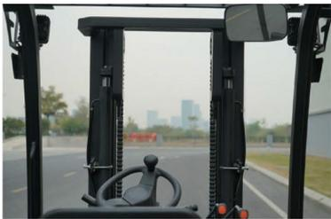
The Q series trucks have a wide visibility mast, offering the operator precision and comfort.
