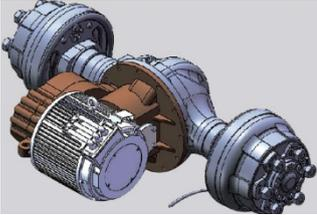
The transmission system uses a horizontal drive axle with a high transmission ratio. The battery is mounted at the bottom of the chassis. The trucks are equipped with a maintenance-free AC motor and a long wheelbase (700 mm) for greater stability.
